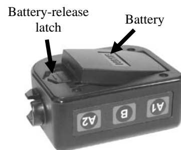
Figure 6. Belt-pac battery-release latch
